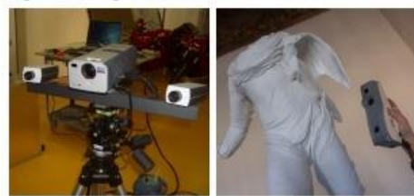
Figure 4. Triangulation laser scanner with structured-light
